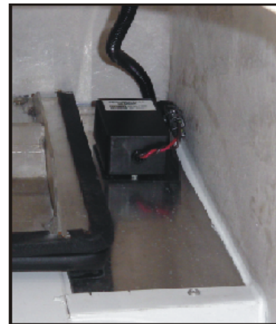
RIGHT: Exterior mounted Temperature sensor (located on front of trailer under the damper scoop)
