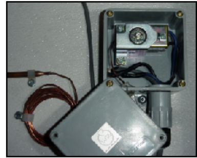
Heater Thermostat – located inside the wall on the curb side of the trailer.
